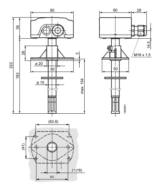
Drilling template with (without) mounting flange
