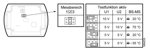
The setting element is located inside the cover. It consists of 6 pins and a shorting plug. It is used to select the required measuring range and to activate the test function.
